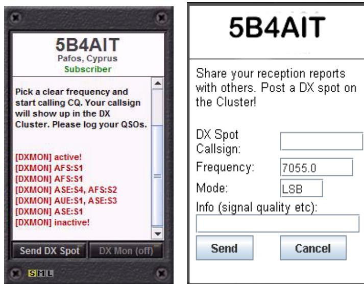
A DX Spot reporting function has been added to the DX plugin. This is where you can send "DX spots" (stations that you receive to let others know that a contact may be possible) directly to the DX-Cluster. Note: The DX Spot comment section is limited to 40 characters.
