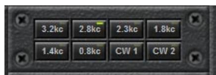
These help filter out unwanted noise whilst receiving. The lower the number, i.e. 1.4kc the more filtering (narrower reception) of the received audio signal. Note that the 800Hz and 400Hz are normally only used in CW/Digi mode.
