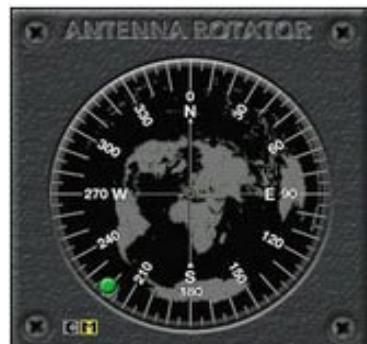
Some of the antennas you purchase are directional and you will need a rotator to “point” them in the desired direction, to achieve this you will need the antenna rotator plugin. There are two views you can have on your rotator that is a compass view (C) or a map view (M). It is worth noting that the map shown on the rotator is a great circle map, centered on your location. Use this link if you wish to generate your own Great Circle Map - [Create an Azimuthal Map](#).
