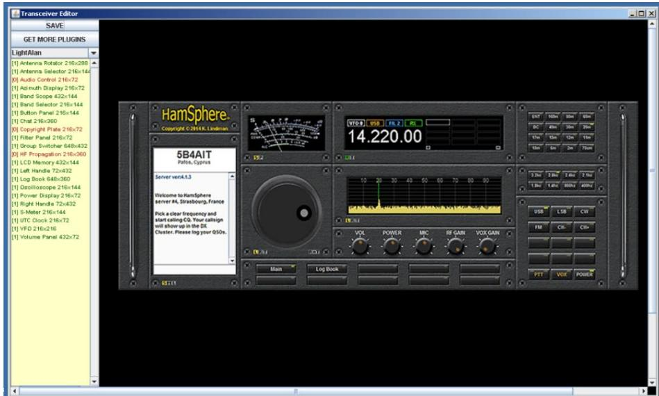
To move plugins around in the editor you need to click near the top edge of the plugin and drag it to the desired location. To remove a plugin from your rig, drag it to the left into the repository. Stored unused plugins will appear in green in this
